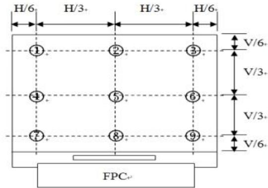
**Note 4:** Definition of Contrast Ratio (CR): measured at the center point of panel
